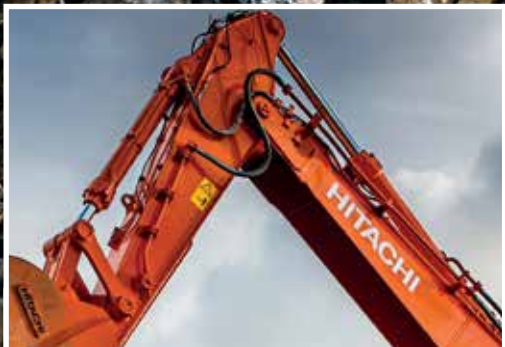
Reinforced boom and front attachment.
