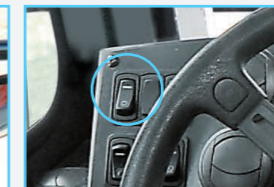
Screen Changeover Switch
