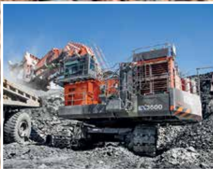
EX ultra-large excavators
