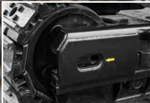
The strengthened motor guard and idler bracket protect against damage.
