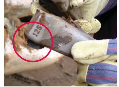
3. Inspect for distorted, damaged, or protruding rubber on the pin body.
