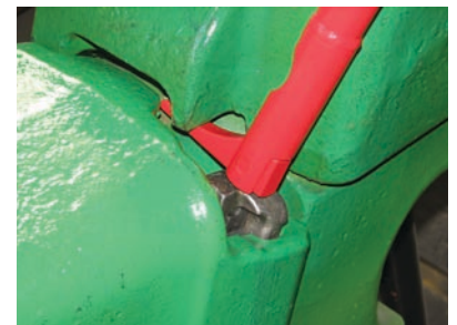
6. Lever the tool to lock pin in place. Often a ping sound occurs when the pin locks in place.
