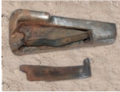
2. Inspect for missing or damaged latch.
