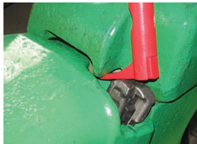
5. Position pry tool. Place pry end of tool under pry tabs in wearcap (if wearcap present) or under the point for non-wearcap assemblies.
