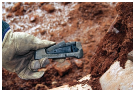
7. Reassemble latch and rubber in pin body.
