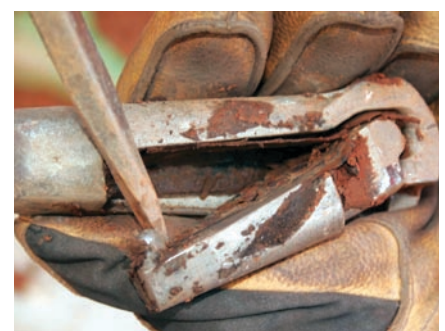
5. If fines have infiltrated the SV2 pin assembly, then disassemble the pin by prying the latch and rubber plug from the pin body.
