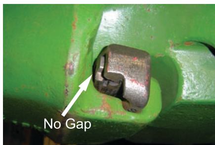
7. Check to ensure lock is bottomed out and latch is fully engaged. When installed, there should be no gap between the pin latch face and the point.
