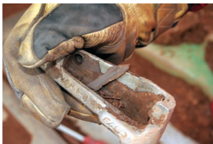
6. Remove the fines from the pin body cavity.
