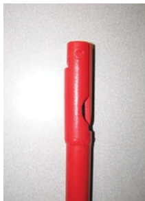
4. The pry end of the tool must be in the open position for pin installation. The pry end must be closed at all other times.
