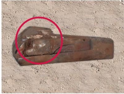
1. Inspect for excessive top wear.
