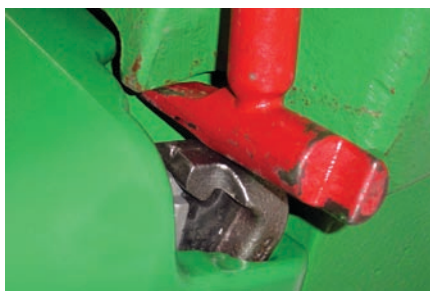
4. Position pry tool. Place pry end of tool under pry tabs in wearcap (if wearcap present) or under the point for non-wearcap assemblies.
