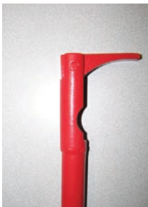
4. The pry end of the tool must be in the open position for pin installation. The pry end must be closed at all other times.
