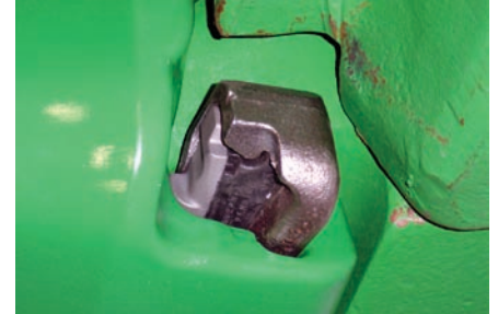
3. Position the SV2 pin. The SV2 pin only installs into the point ear in one direction. Failure to position pin correctly can lead to pin and point loss.
