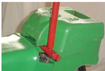
5. Lever the tool to lock pin in place. Often a ping sound occurs when the pin locks in place.
