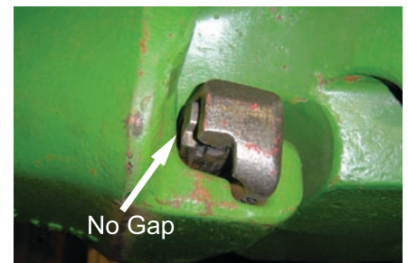
6. Check to ensure lock is bottomed out and latch is fully engaged. When installed, there should be no gap between the pin latch face and the point.
