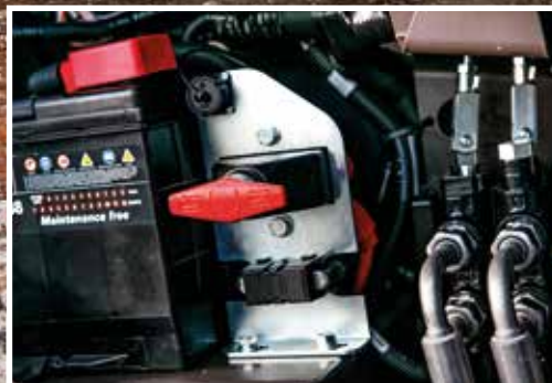
Battery disconnect switch for easy maintenance.
