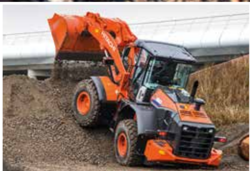
The optional belly guard provides added protection.
