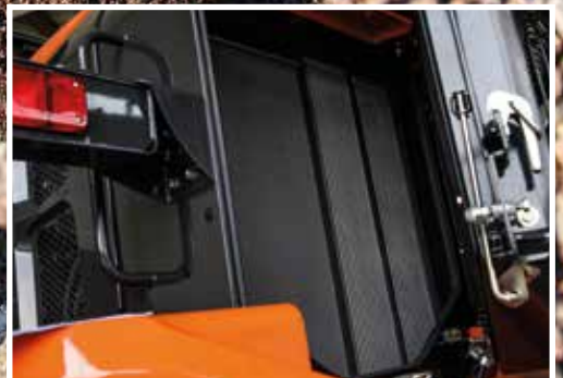
Optional anti-clogging radiators enhance durability.
