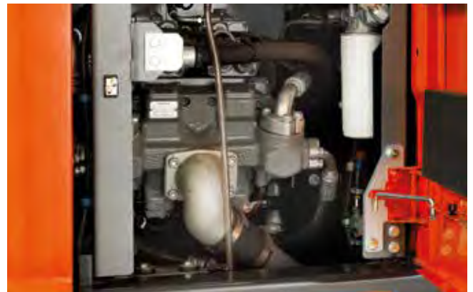
A fuel saving of up to 5% is achieved with the HIOS V hydraulic system (ZX150W-7 and ZX155W-7).
