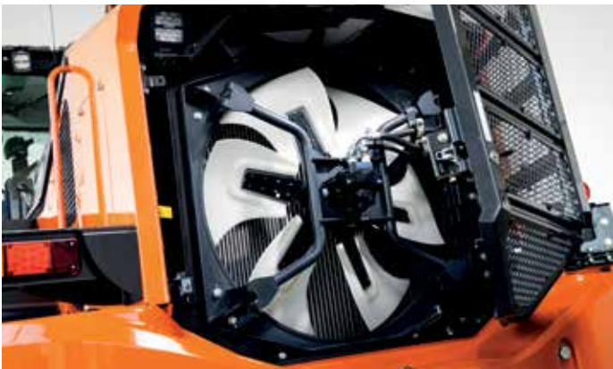
Intelligent fan operation system prevents radiators clogging.
