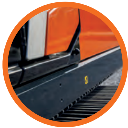
The upper structure has side protection and a reinforced underside for additional robustness.
