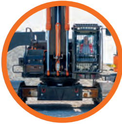
The triple boom cylinder enhances versatility.
