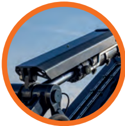
Bucket cylinder protection designed for challenging working conditions.
