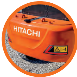
Additional counterweight provides added stability.
