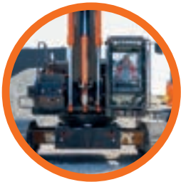
The triple boom cylinder enhances versatility.
