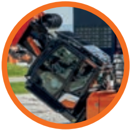
Excellent visibility thanks to the tilting cab (to an angle of 30 degrees).
