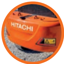
Additional counterweight provides added stability.
